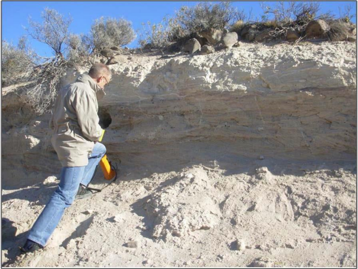
Figure 3.15: Typical prospective unit – ‘dirty’ sandstone unit sandwiched by basal white tuff and overlying sandstones and calcrete
